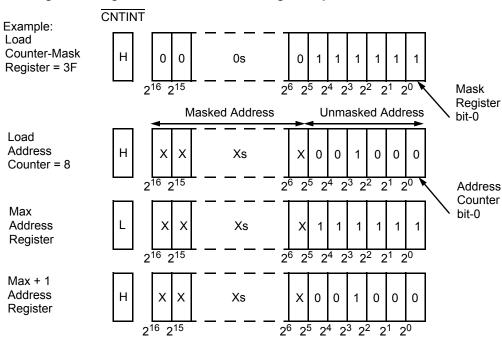
Figure 3. Programmable Counter-Mask Register Operation[1, 22]
